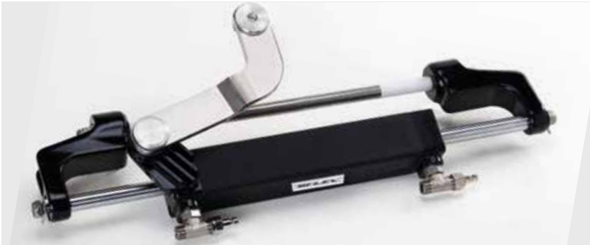
UC94-OBF/3 - Balanced: the number of turns lock-to-lock is equal port to starboard or vice-versa
