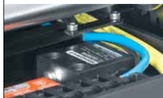
Two inner magnetic switches factory-set at the feeder's stroke limits prevent overtravel. Two outer fail-safe limit switches automatically engage the brake.
