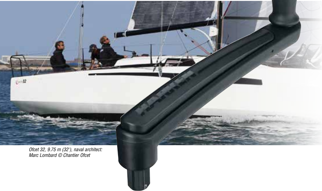
The patented locking mechanism features two stainless steel pins that automatically retract when the handle's full-length grab bar is squeezed, and extend when it is released for a solid, secure lock.
