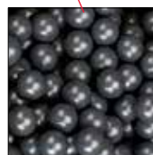
Delrin® UV-stabilized: Ball bearings
