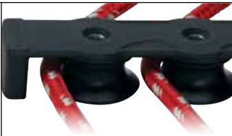
Asymmetrical sheaves lift lines off deck.
