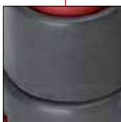
6061-T6 aluminum: Hard Lube-anodized
