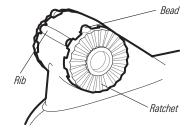
Fitting the Mounting Bracket over the Ratchet
