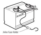
**CAUTION:** Some boats have 24 or 36 Volt electrical systems. Make sure that your HDR 650 is connected to a 12 VDC power supply. Use a voltage conditioner for variable inputs.
