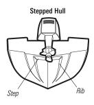
**Turbulence:** You must first determine the best location on the transom to install the transducer. It is very important to locate the transducer in an area that is relatively free of turbulent water. Consider the following to find the best location with the least amount of turbulence:
