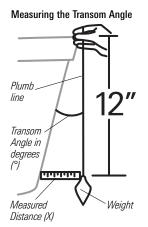
1b. If you do not know your transom angle, measure it using a plumb line (weighted nylon string or monofilament line) exactly 12 inches long. Hold the top of the plumb line against the top of the transom with your finger, and wait until the line hangs straight down. Using a ruler, measure the distance from the bottom of the plumb line to the back of the transom, then use the chart.
