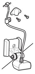
2a. If you are routing the cable over the transom of the boat, secure the cable by attaching the cable clamp to the transom, drilling 9/64" diameter holes for #8 x 5/8" wood screws, then skip directly to procedure 5, *Connecting the Cable*.
