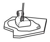
Press the transducer into place with a slight twisting motion to purge any trapped air from underneath, keeping the pointed end of the transducer body pointed forward, towards the bow (see the illustration *Pressing the Transducer Into Place*).
