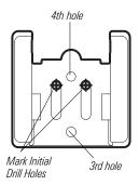
3. Continue to hold the bracket on the transom of the boat, and use a pencil or marker to mark where to drill the two mounting holes. Mark the drill holes near the top of each slot, making sure that your mark is centered in the slot (see the illustration *Using the Mounting Bracket to Mark the Initial Drill Holes*).
