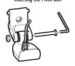
3. Put the pivot bolt through the assembly to hold it in position and loosely install the nut, but do NOT tighten the nut at this time (see the illustration *Inserting the Pivot Bolt*). Insert the pivot arm assembly into the mounting bracket (see the illustration *Inserting the Pivot Arm Assembly Into the Mounting Bracket*). Do NOT snap the assembly closed, as you will need to access the mounting bracket in the next step.
