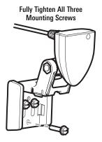
8. Re-position the transducer assembly against the transom of the boat, then hand-install all three screws. Make sure that the transducer location and the pivot angle have not changed, then fully tighten all three mounting screws (see the illustration *Fully Tighten All Three Mounting Screws*). Snap the pivot back down. If you have performed the preceding procedures correctly, the transducer should be level and at the right height for optimal operation.
