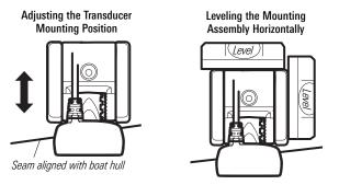
**NOTE:** The deeper the transducer is in the water, the more likely that a rooster tail of spray will be generated at high speeds, so make sure that the transducer is as high as it can be and still be submerged in the water.
