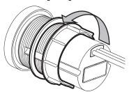
3. Hand-tighten the collar until the HDR is securely mounted in the dashboard. Make sure that the face of the HDR stays oriented upright.
