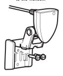
Align the mounting bracket transducer assembly with the drilled holes in the transom. With a 5/16" socket driver, mount the assembly to the transom using the two #10 - 1" long screws provided (see the illustration Mounting the Assembly to the Transom).
