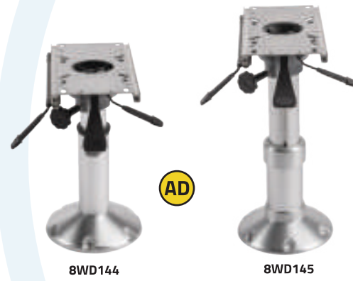
8WP144 STANDARD MAINSTAY PEDESTAL Features Air Powered Adjustment: 14" to 20" 2 3/8" Diameter Post, 9" Anodized Base Locking Seat Mount w/ Fore & Aft Slide Ideal for Freshwater Helm Seat Applications 8WP145 Heavy Duty Mainstay Pedestal 2 3/8" Diameter Post, Ideal for Saltwater Helms
