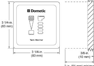
2-in. (51 mm) minimum clearance behind wall
