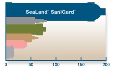
Chart indicates calculated capacity in grams of carbon disulfide that are adsorbed by each laboratory-tested\* vent filter. Based on this data, SeaLand SaniGard vent filters will outlast competitive filters by factors of 2.4 to 12.6 times longer. \* Vent filter tests conducted by Intertek Group, Chicago, IL, USA.
