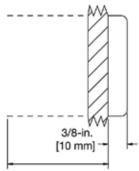
2-in. [51 mm] minimum clearance behind wall
