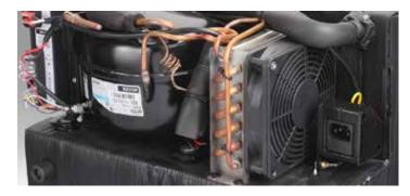
Unique to the CRX series, the speed-controlled compressor runs at mid speed when starting up, switches to high speed for temperature pull down, then runs at low speed while maintaining the set point. The result is a quieter unit that runs more efficiently. The tube-and-fin condenser provides greater performance, durability, and corrosion resistance over the traditional static condenser. The large fan provides better cooling performance, especially in high ambient temperatures.
