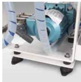
Vibration-isolation mounts reduce noise and vibration.
