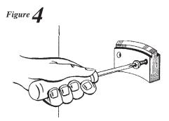
4. Install Mounting Bracket. Position black Mounting Bracket on the inside wall of the sink cabinet. Use the two Self-Tapping Screws to securely install the Bracket. Make sure the Bracket location permits access to the cold water valve location and easy access for Cartridge changes.
