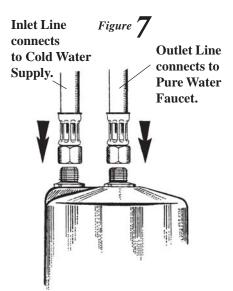
8. Connect Inlet and Outlet lines. Connect free end of Thermoplastic Connection Hose from Faucet Stem to Outlet (center) Port on the Pressure Vessel. Tighten securely. Do not overtighten. Connect remaining Hose from fitting on cold water supply line to Inlet (outside) Port on top of Pressure Vessel. Do not overtighten.
