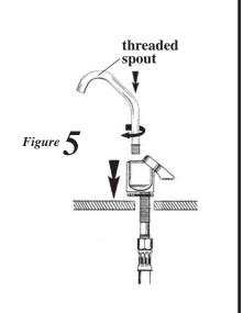
6. Connect Hose directly to Faucet Stem and tighten securely by hand. Do not overtighten. Insert and thread Spout into base, Do not over tighten (figure 5). Drop free end of Connector Hose through previously prepared hole and position Faucet in hole.
