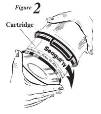
Install Cartridge. Thread Cartridge (Fig.2) into top half of Pressure Vessel (Be careful not to cross thread.) until contact is first made with Rubber Seal. Then tighten ¼ turn only. Do not overtighten. Be sure Pressure Vessel Flanges and Housing Gasket are clean and free of dents, nicks or cuts.
