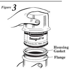
**3. Reassemble Pressure Vessel.** Place Gasket on Flange of lower half of Pressure Vessel (Fig.3) and reassemble V-Clamp, keeping Seagull IV logo upright. The Wing Nut on the Clamp should be tightened snugly, by hand only. *Use no tools to tighten.*
