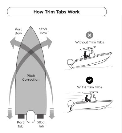
When the tabs are deployed downward, the water force on the trim tab surface creates upward pressure, raising the stern and lowering the bow. The port trim tab lowers the starboard bow, and the starboard trim tab lowers the port bow.
