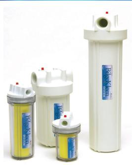
The patented BilgeKleen System automatically removes oil, gas, diesel fuel and other hydrocarbon pollutants from bilge water before it is discharged overboard. Using a special filter medium, the BilgeKleen captures and binds to hydrocarbons and lets water pass through freely. As a result, 99.9% of the hydrocarbon pollutants are eliminated from discharge with no increase in pressure to the bilge pump.
