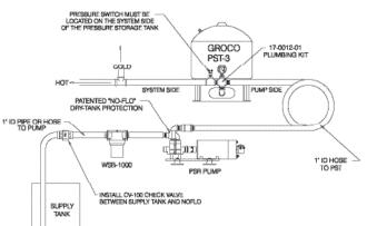
**PLUMBING:** Fasten 17-0012-01 plumbing kit onto the PST (pressure storage tank) with the pressure switch on the system-side of the PST and the hose barb on the pump-side of the PST as shown above. To aid in initial priming, pour water into the pump inlet before connecting hoses to the pump. Plumbing between the pump and the PST must be 1" ID heavily reinforced hose, and must be free of valves, filters, or any other device. Plumbing after the PST may be reduced.
